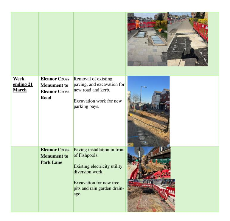
Park Lane to northern end of the High Street (adjacent to Wickes) Continued drainage works and excavation for kerb braces, new road alignment, parking bays and footpath concrete foundations.
