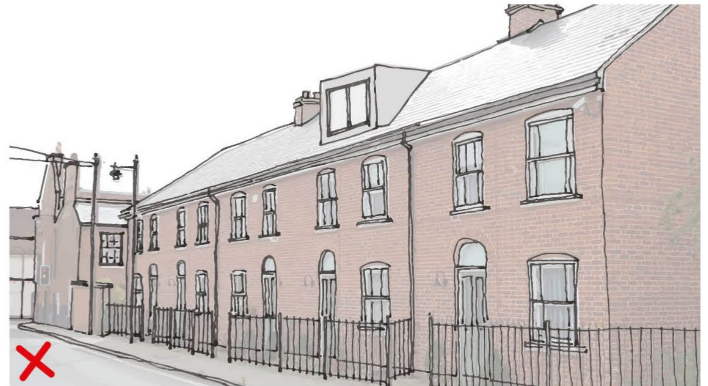
A front dormer on this row of terraces breaks the strict geometry of the facade and roof form and impacts negatively on the streetscene.
