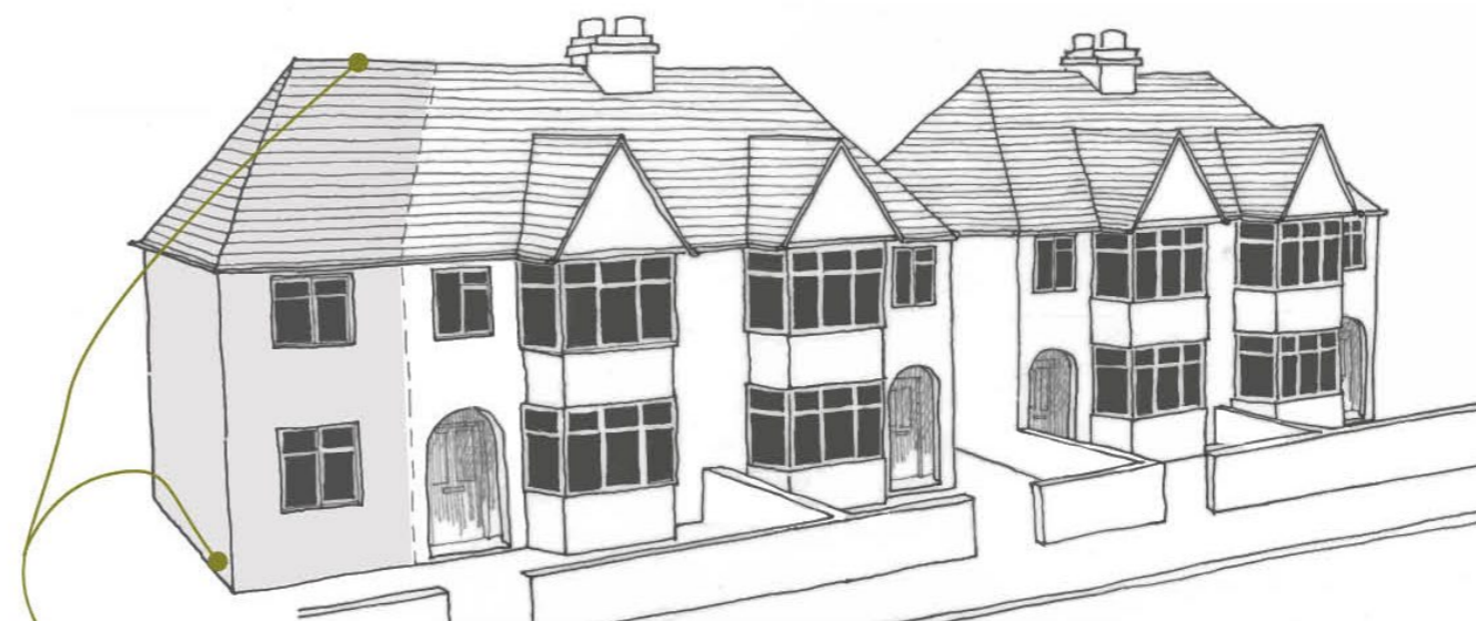
This large side extension with matching roof ridge lines and front aligned with the line of the front facade is unacceptable because it makes the house look unbalanced and lopsided.
